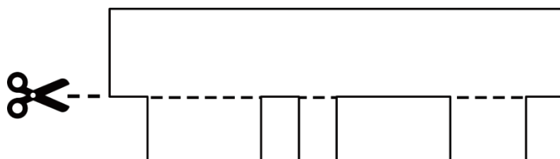
Fig. 6 - Starting row preparation
