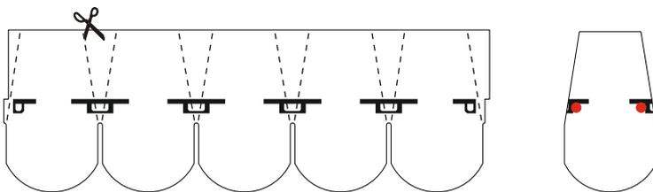
Fig. 7- Cutting of the ridges
