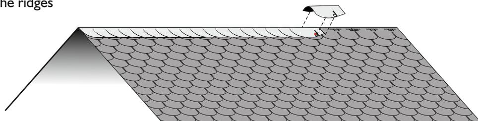
Fig. 8 Installation of the ridges
