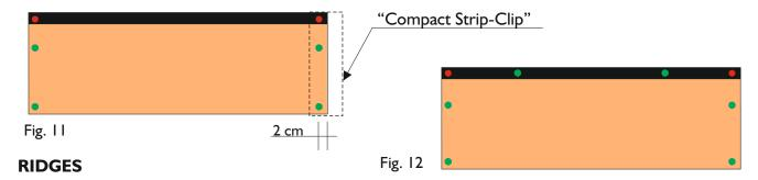
Install COMPACT shingles on both sides of the roof till the ridge line and cut the shingle which overshoot the ridge.
