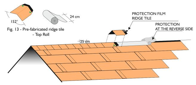
Fig. 14 - installation of the ridge tiles
