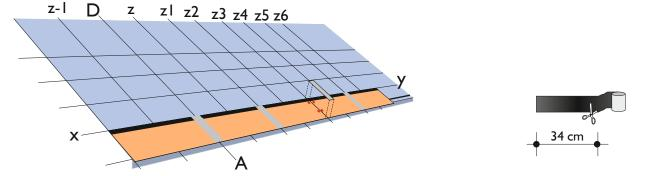
Fig. 6 - Installation of Compact Strip
