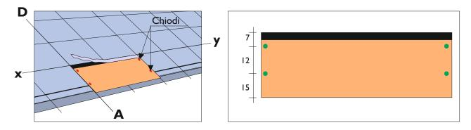
Fig. 4 - Installation of the first shingle Compact
