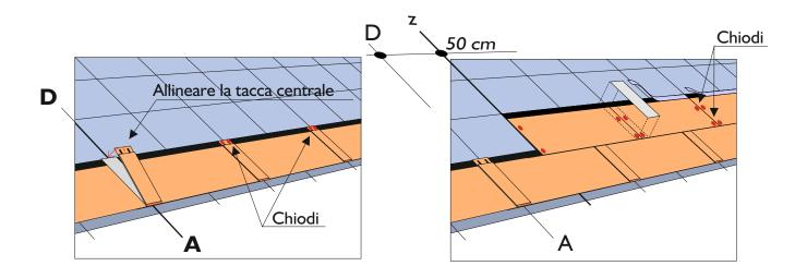
Fig. 8 - Installation of Compact Clip
