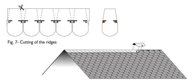
Fig. 8 Installation of the ridges
