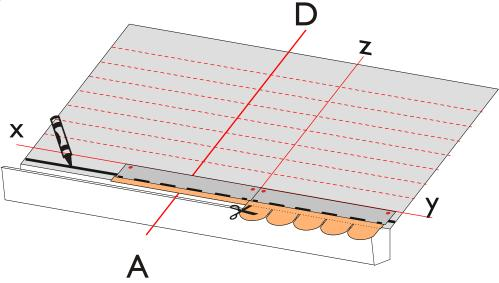
Fig. 3 - Installation of the starter course
