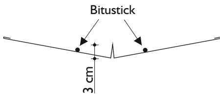
Fig. 16 - Flashing (example)
