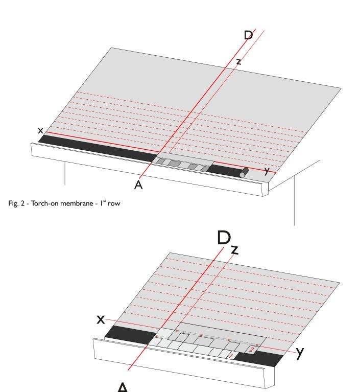
Fig. 4 - Sequence of 2 shingles
